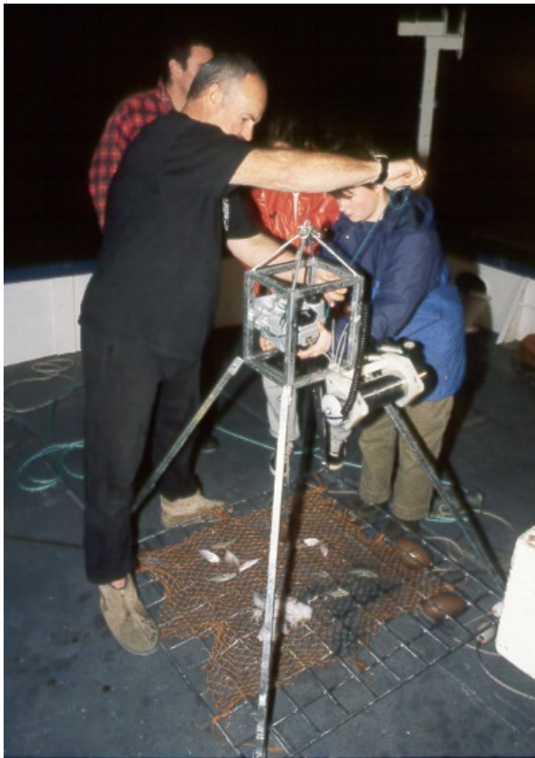
Figure 8.1. Video-camera rig used for cafeteria experiments.
