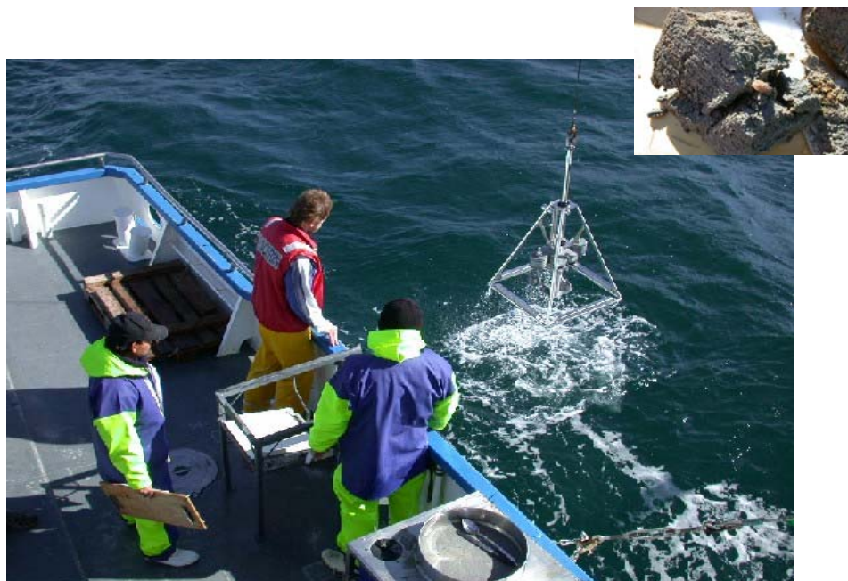
Figure 10.2. Sediment samples collected by using a HAPS corer operated on the research vessel Ngerin. Inset: the coarse sediment collected by the corer at a control site.
