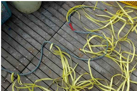
Figure 9. Joint venture vessel tori line streamers.
