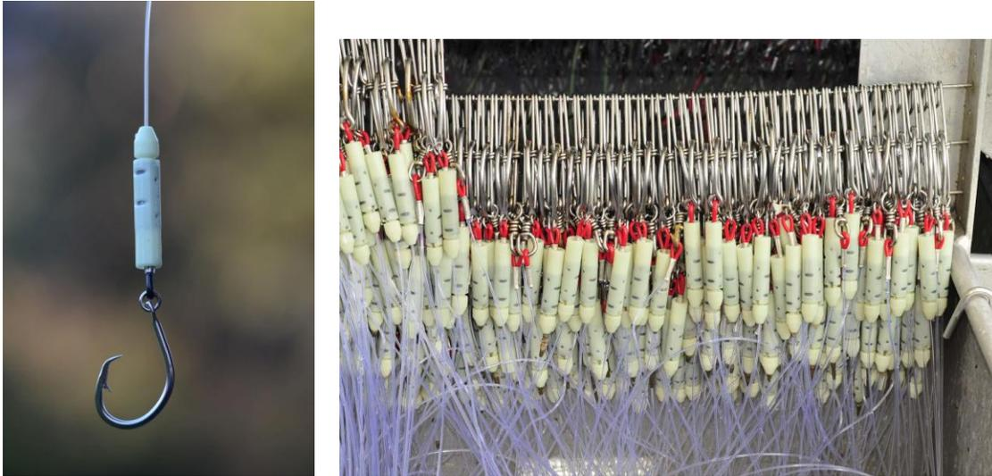
*Figure 2. A 40 g hook weight and a # 14/0 circle hook showing the luminescent nylon coating and its position on the branch line (left). The lower one-third of the lead is rebated to fit over the crimp. The photo on the right shows 40 g weights attached to layers of branch lines in a gear bin.*
