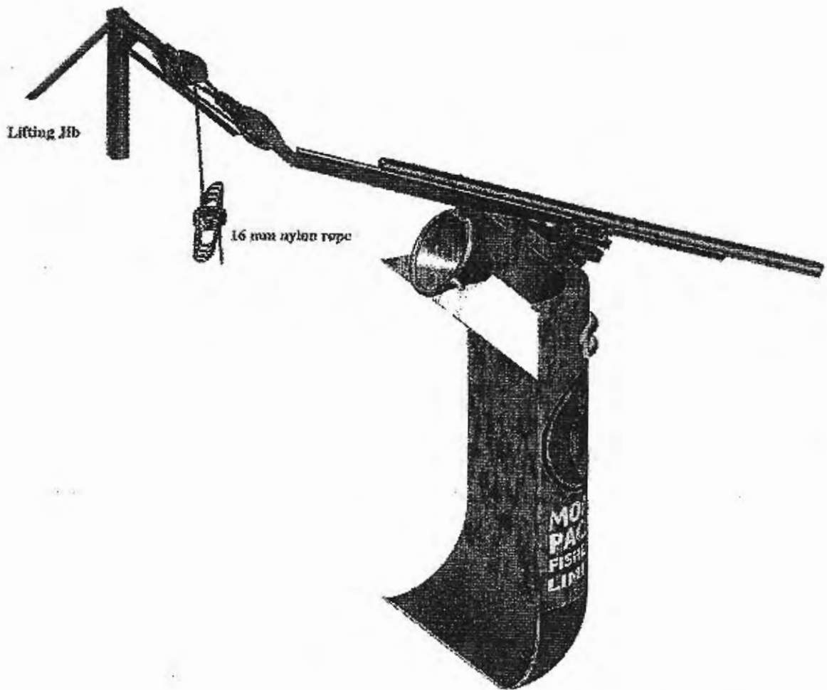
FIGURE 16. SECOND METHOD OF DEPLOYMENT AND RECOVERY OF THE CHUTE TRIALED ON F.V. ATU S.
