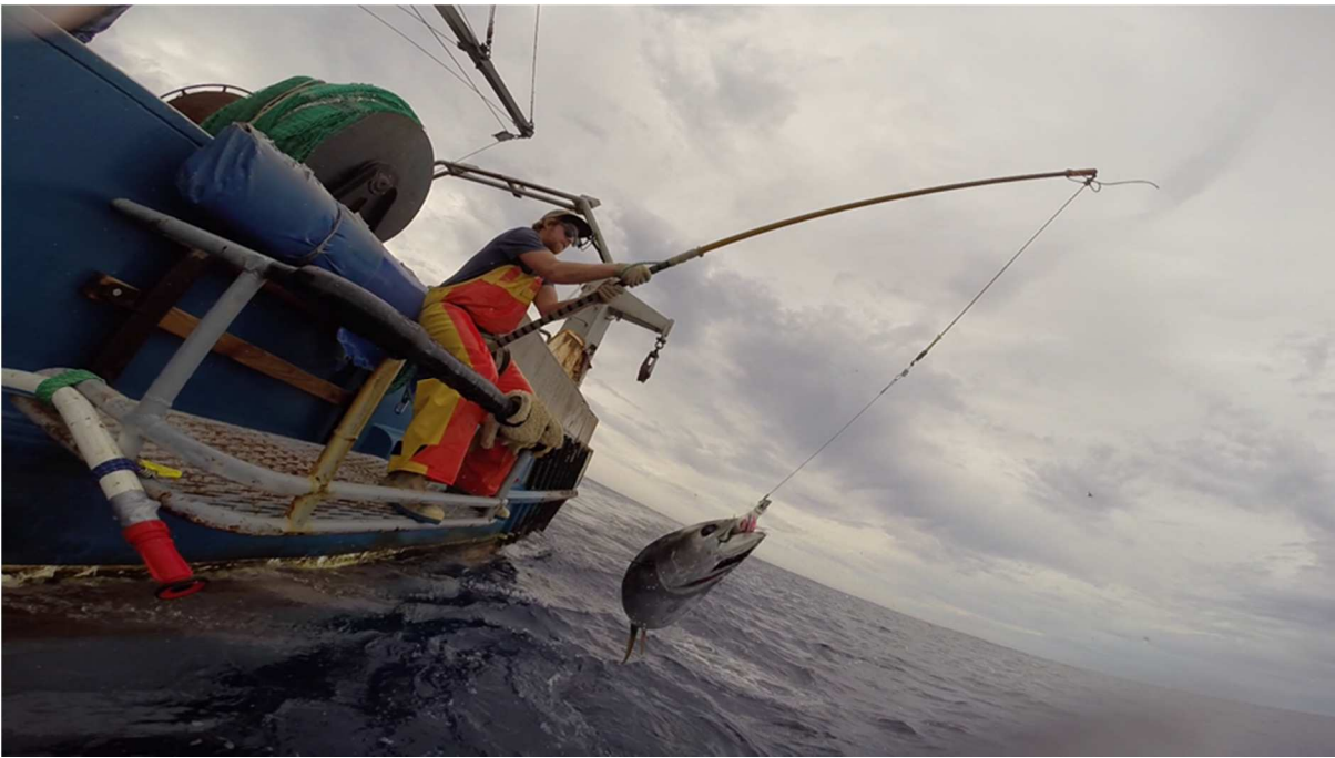
Figure 5: Single -person poling rack on port side of FV Celtic Rose for the capture of SBT (photo: R. Bradford).
